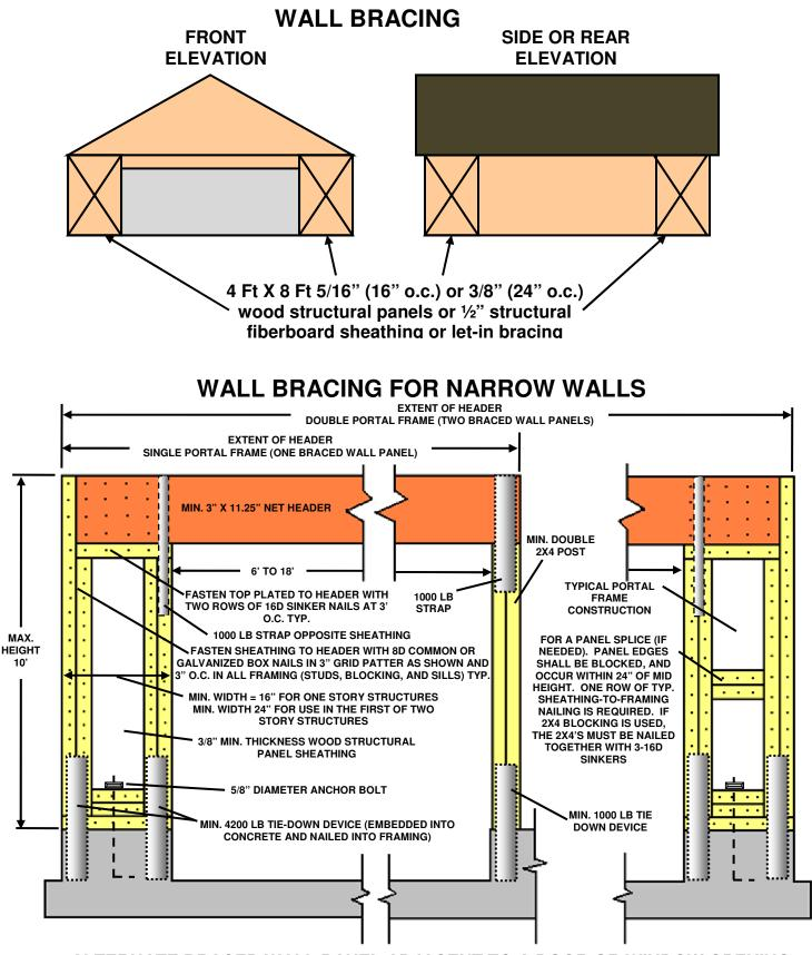
ALTERNATE BRACED WALL PANEL ADJACENT TO A DOOR OR WINDOW OPENING
